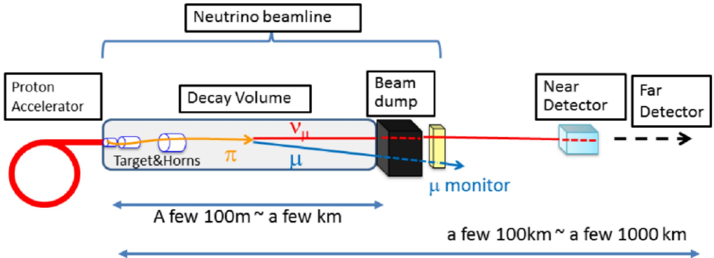
**FIGURE 1.** Components of the accelerator neutrino experiment
