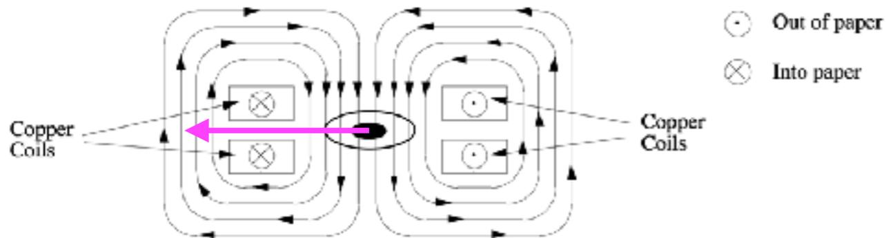
To make the beam travel in a circle it is deflected by dipole magnets.
