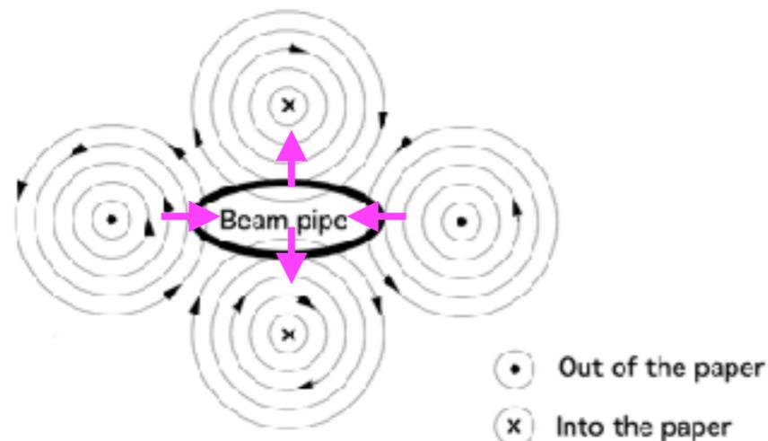
To keep the beam inside the pipe, it is squeezed in the vertical and horizontal directions by quadrupole magnets
