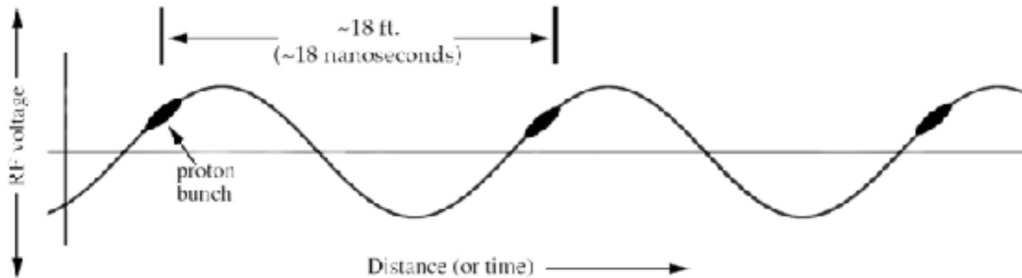
Beam is accelerated by applying a pulsed electric field; 56 MHz "Radio Frequency", RF. The beam naturally falls into the minima of these "buckets"
