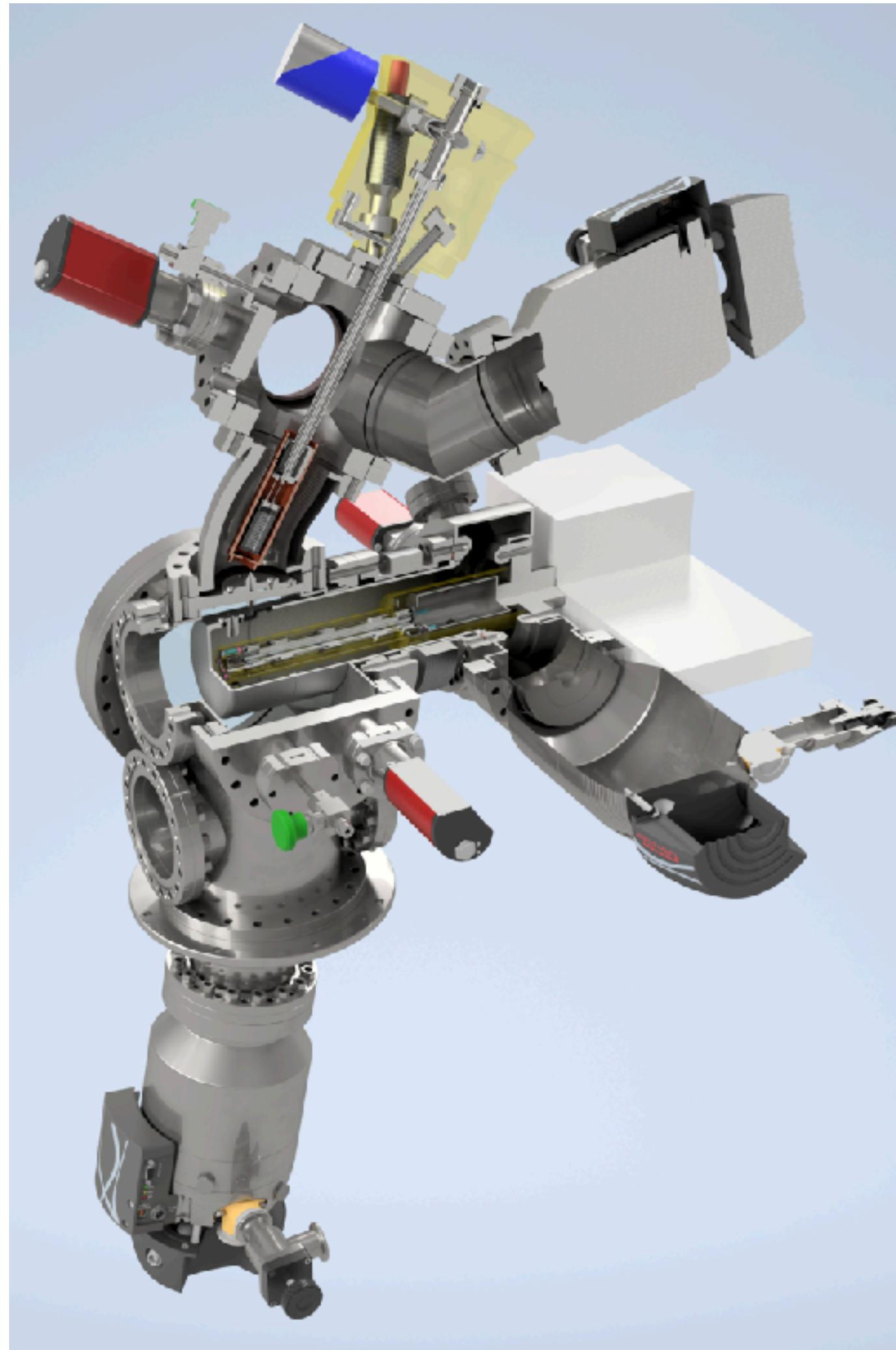
Setup for atomic hydrogen production
