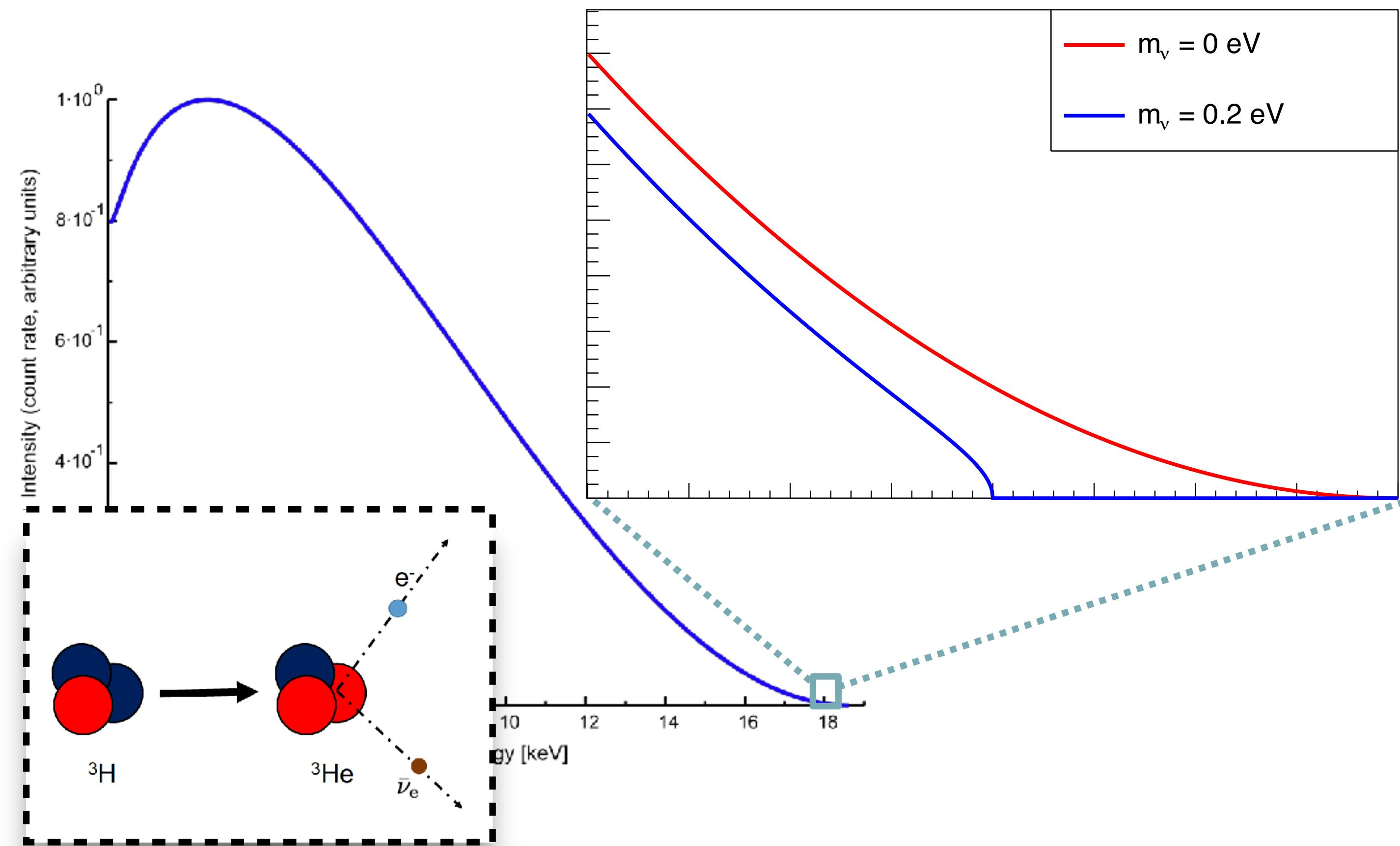
$$\frac{dN}{dE} = K \underbrace{|M|^2}_{\text{Matrix element}} \underbrace{F(Z, R, E)}_{\text{Fermi function}} p_e E (Q - E) \sqrt{(Q - E)^2 - \boxed{m_\beta^2}}$$
