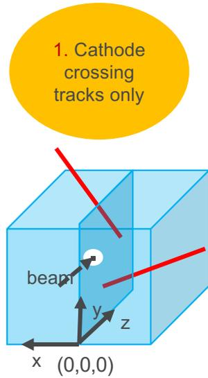
Position along the drift direction is only accurate for cathode crossers
