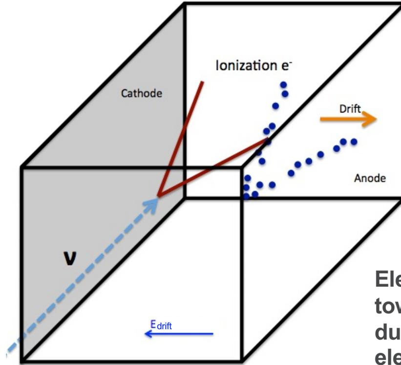
Electrons drift towards anode due to applied electric field
