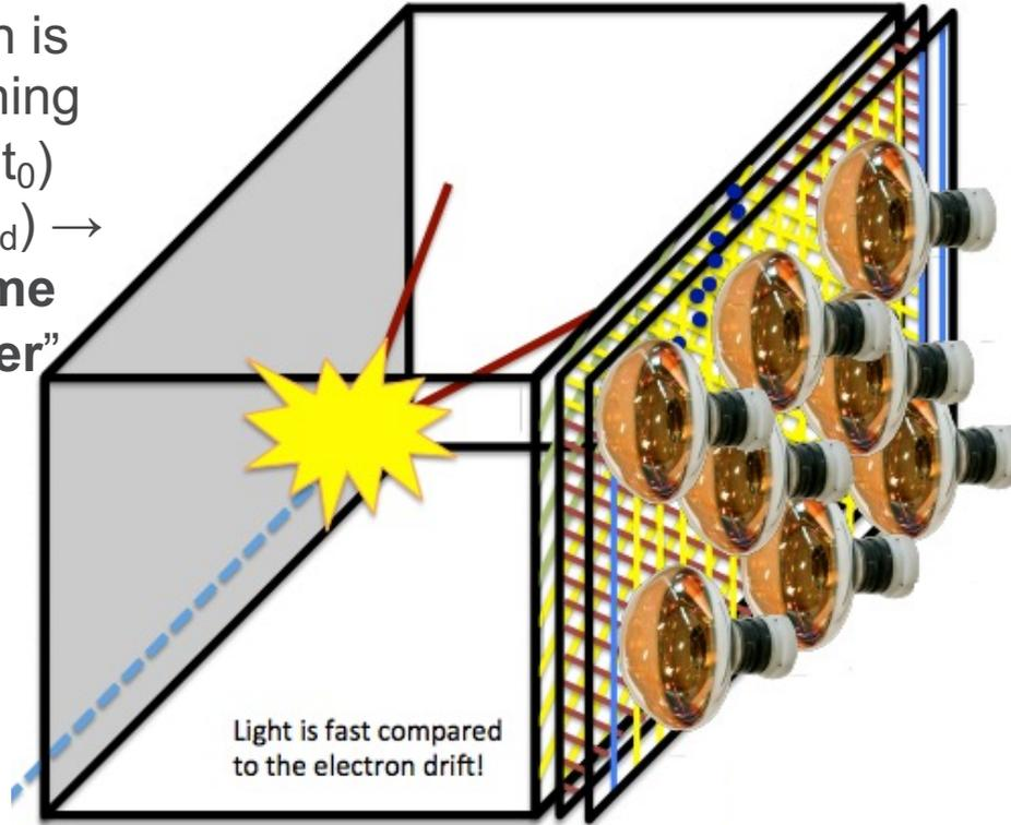
**Scintillation light is collected by PMTs that give absolute time for the interaction**
