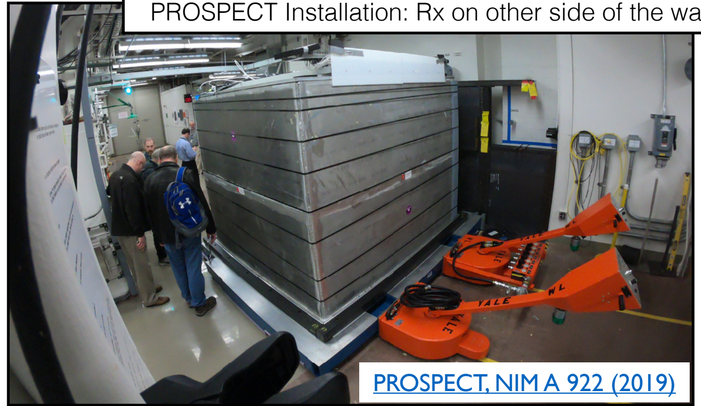
PROSPECT Assembly: adding top row of segments
